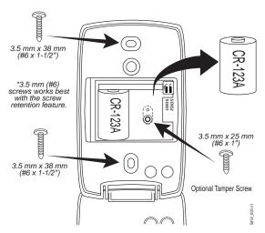
\*The screw retention feature simplifies installation: A rib in the screw cavity lightly holds the screw in place when installing the detector.
